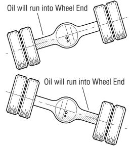
Fill Housing with oil to bottom of Plug
