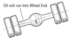
3. Raise the right side of the axle 6 in. [152 mm] or more. Hold axle in this position for one minute.
